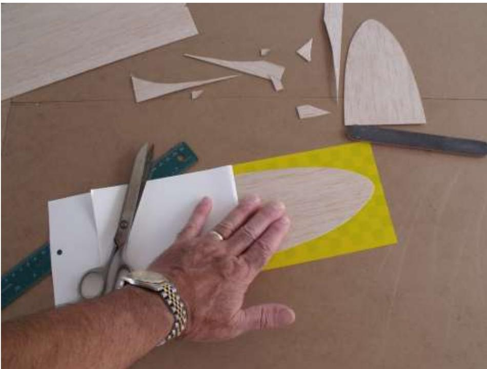
After folding the Monokote onto the opposite side, I cut the excess Monokote off the SFG.
