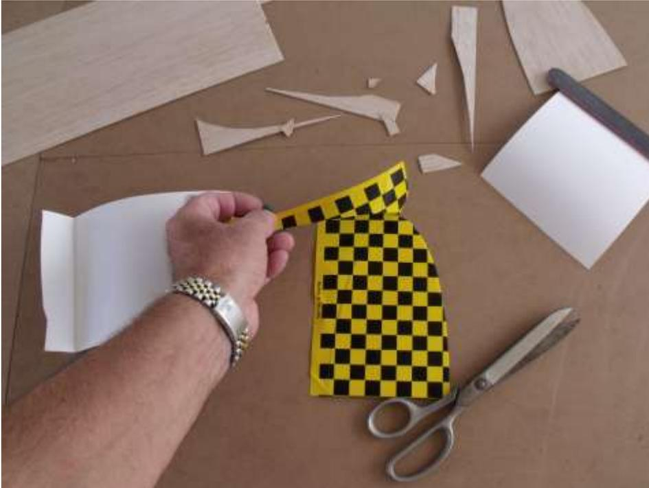
In order to make sure my Monokote would not peel back in flight, I decided to use ¼ inch trim tape to seal the edge.
