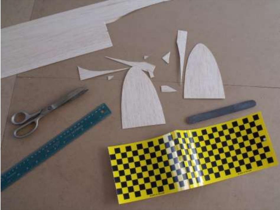
The next step was to cut the Monokote to fit the one SFG, and fold it down the middle so that I could fold the Monokote over the straight trailing edge.
