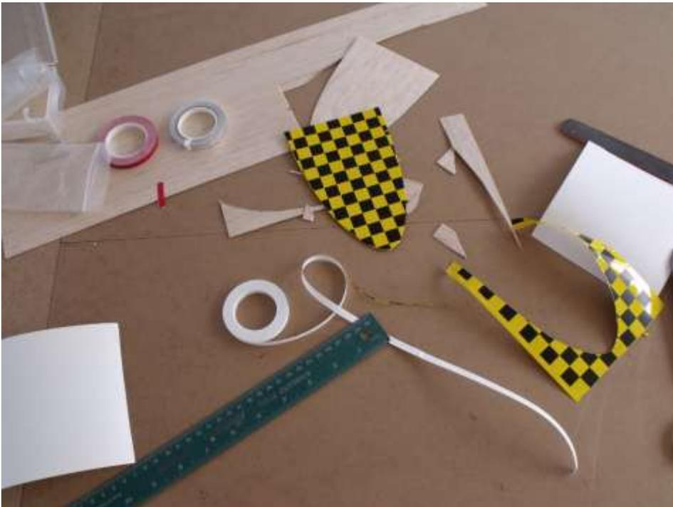
The white trim tape I used is very elastic and fit perfectly around the curved surface.
