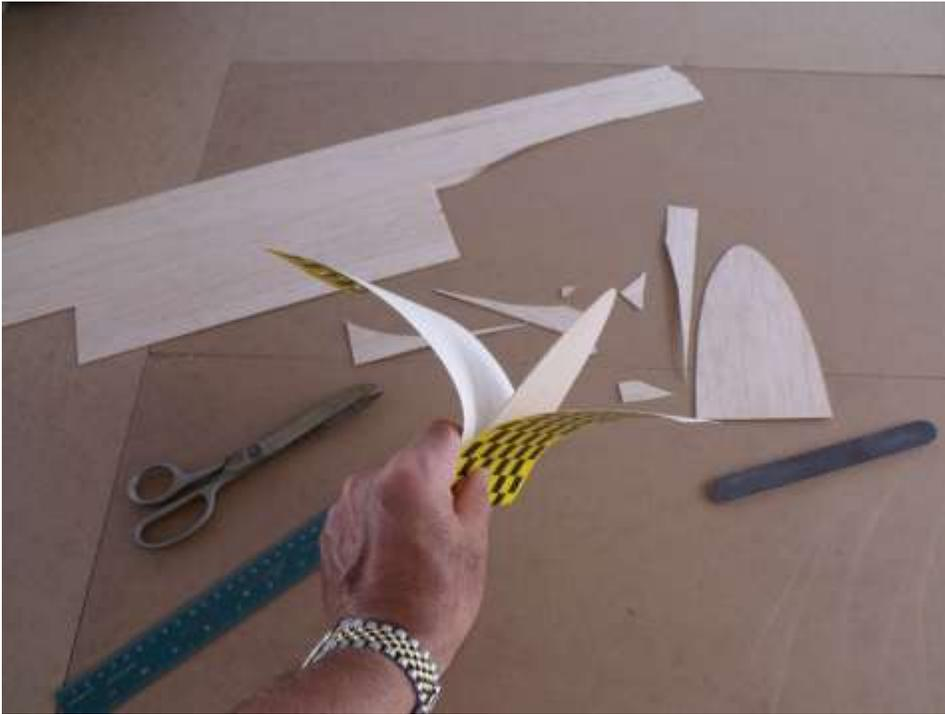
I peeled back the paper on the adhesive side, laid the Monokote flat on the workbench, and pressed the balsa SFG in place.
